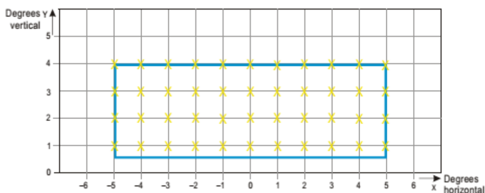
Figure A2-21. Grid points to be used for calculation of average intensity of taxiway centre line and stop bar lights
